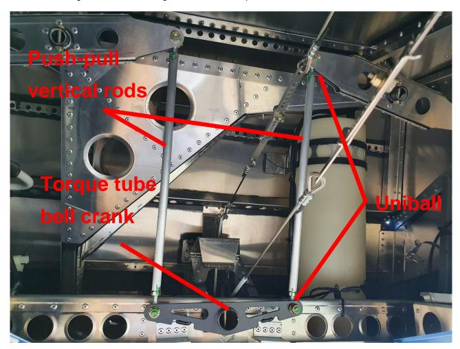
Figure 42: Push-pull rods for Flaperon setup
