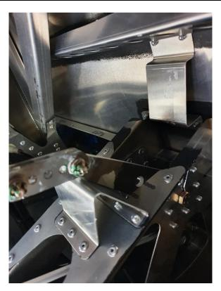
Figure 44: Longitudinal line bell crank on the full nose up position, against stop
