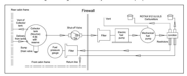
Figure 27: Fuselage and Rotax 912 UL/ULS fuel system
