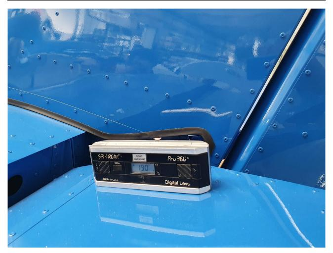
Figure 46: Elevator final setup deflection angle
