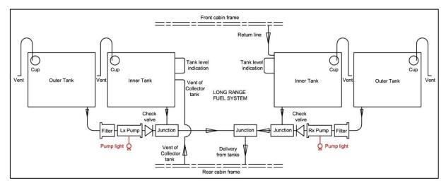
Figure 26: Wing double fuel tank system with transfer pumps
