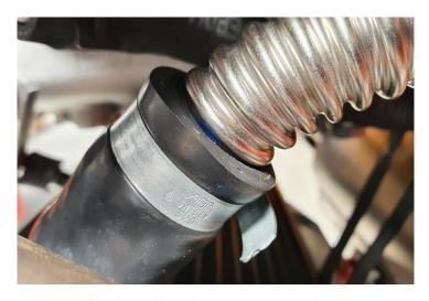
Figure 9: Water hose on corrugated pipe
