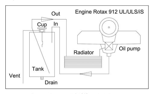
Figure 29: Rotax 912 UL/ULS/iS standard oil system
