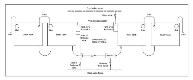
Figure 25: Wing double fuel tank system (interconnected tanks)
