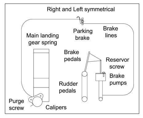
Figure 34: Brake system with parking brake (only right side is shown, the left is identical, symmetrical)
