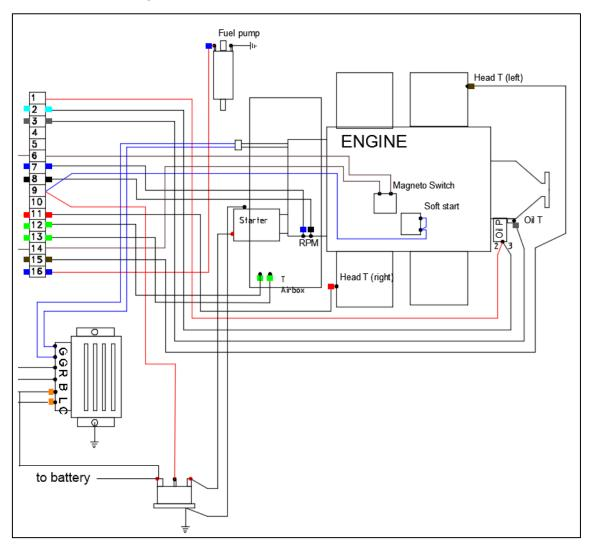
Figure 37: Electrical wiring of engine compartment
