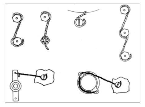
Figure 1: Safety wires example
