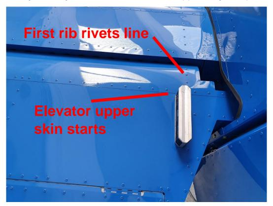
Figure 45: Digital spirit level position on Elevator
