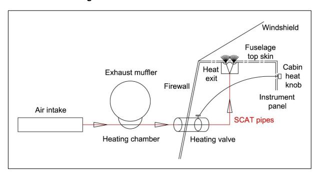
Figure 36: Cabin heating system
