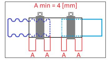
Figure 6: Drawing of connection of hoses on corrugated pipes
