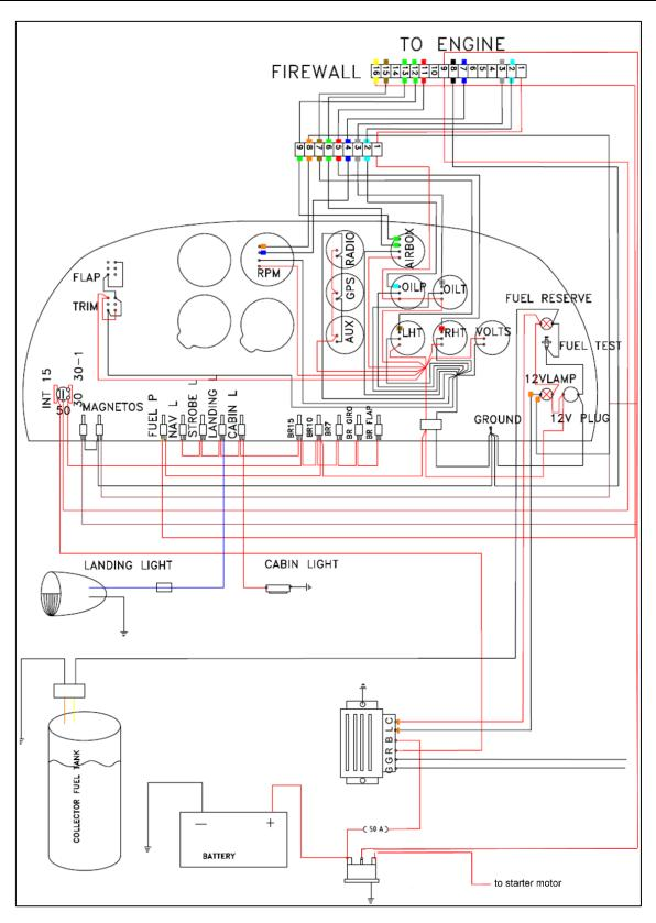
Figure 38: Electrical wiring firewall backward
