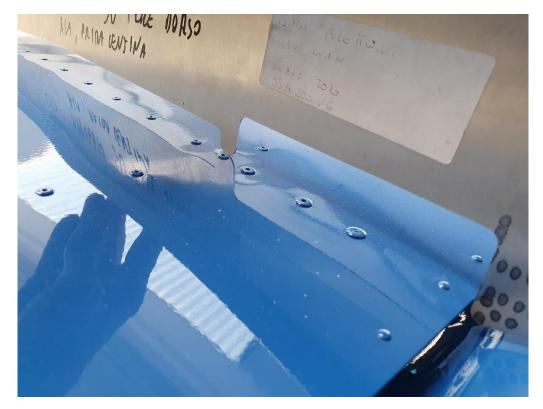
Figure 40: Position of jig SA200VG near the first rib rivets line, aligned to wing trailing edge
