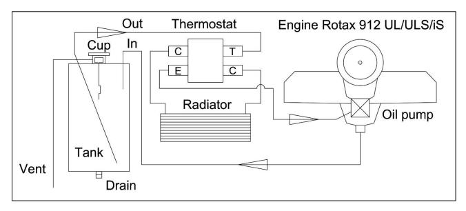
Figure 30: Rotax 912 UL/ULS/iS oil system with thermostat
