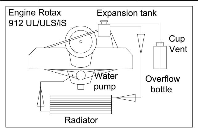
Figure 31: Rotax 912 UL/ULS/iS standard cooling system
