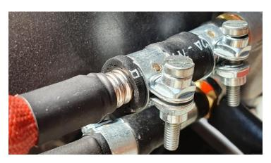
Figure 7: Fuel hose on corrugated pipe
