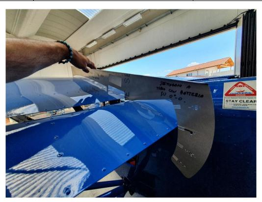
Figure 39: Flaperon jig SA200VG and position on the first wing rib
