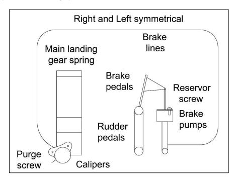
Figure 33: Standard brake system (only right side is shown, the left is identical, symmetrical)
