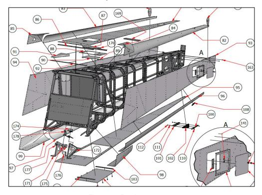
Figure 13: Fuselage rear cone
