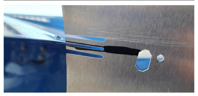
Figure 41: ZERO setting of the left inner Flaperon. Marks of +/- 0.5° of tolerance
