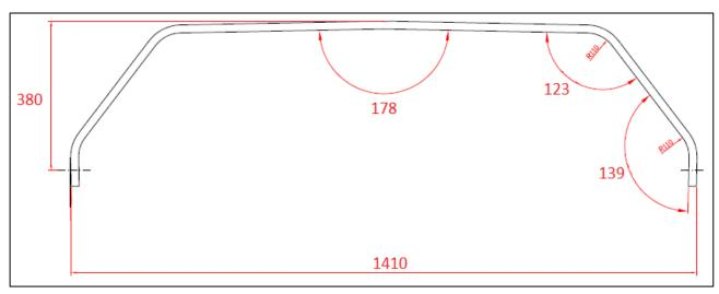
Figure 11: Main landing gear spring design nominal dimensions (unloaded)
