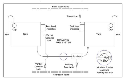
Figure 24: Wing standard fuel system
