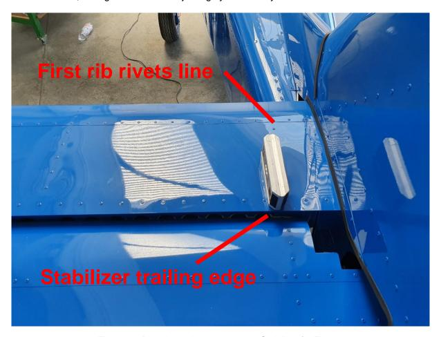
Figure 43: Digital spirit level position on Stabilizer for Zeroing
