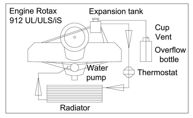
Figure 32: Rotax 912 UL/ULS/iS cooling system with thermostat
