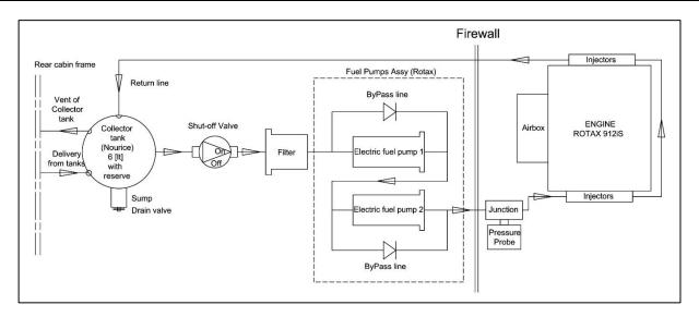
Figure 28: Fuselage Rotax 912 iS fuel system
