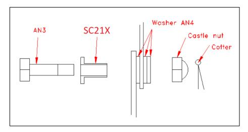
Figure 47: Control surfaces hinges
