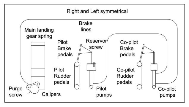
Figure 35: Double side brake system (only right side is shown, the left is identical, symmetrical)
